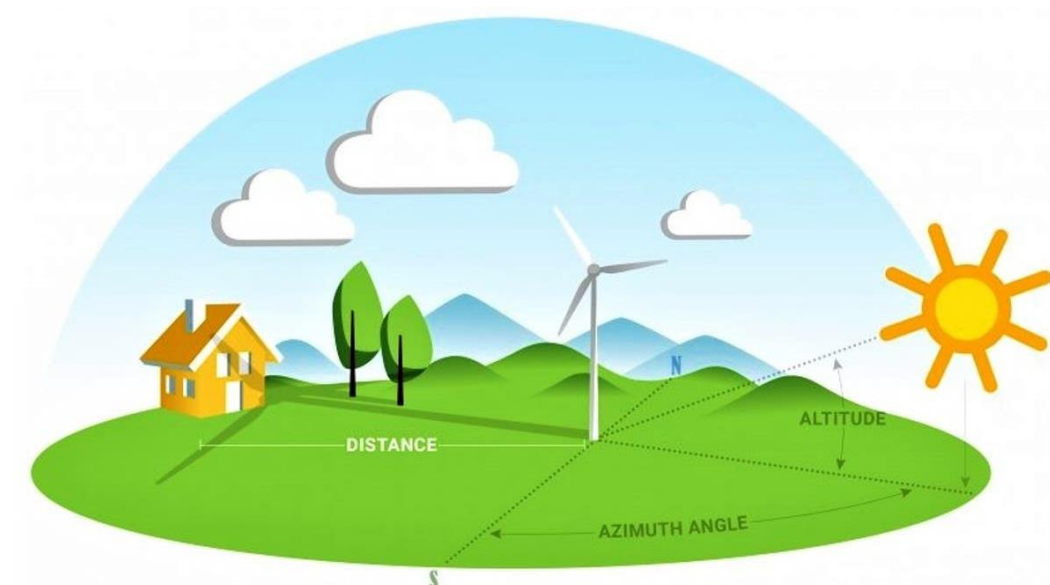
Figure 14.11 Explanation of Shadow Flicker - based on CleanTechnica Figure
